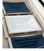
The glass sheet is put on STEP 3 a special mold and put back in the kiln for 24 hours. This is where it is slumped to the sink form.
