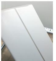
Multiple pieces of glass STEP 1 are cut and carefully stacked. The size and shape of the sheets will determine the final size of the sink being created.
