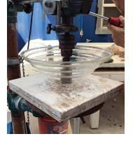
STEP 5 The glass sink is cold worked while at room temperature. A diamond bit drill and sander are used to create the drain hole.
