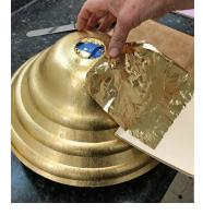
STEP 6 Metal leaf is hand applied once the glass surface has been coated with an adhesive. The leafing is gently tapped into place then brushed for even application.
