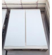
The glass sheets are STEP 2 heated in a kiln to fuse them into a single sheet. The heating strengthens the glass making it 5-7 times stronger than normal unheated glass.
